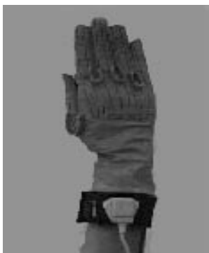
Figure 2 A data glove with eighteen sensors.
