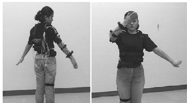
Figure 1 Motion capture with sixteen sensors, and a pair of wired data gloves with eighteen sensors.
